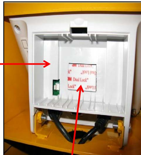
Battery removed revealing Velcro Pad. Tape should be removed from pad to expose stick surface. Battery Pack should be pressed against sticky surface.
